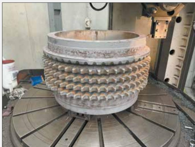
The sprocket assembly before spraying shows clear signs of wear and pitting on the bearing surface.
