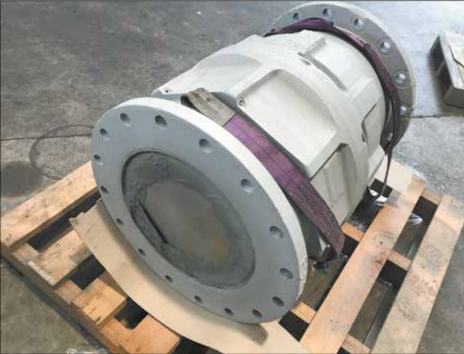
This breakaway housing has been zinc metal sprayed. The surface coating offers greater and longer lasting protection than conventional galvanising.
