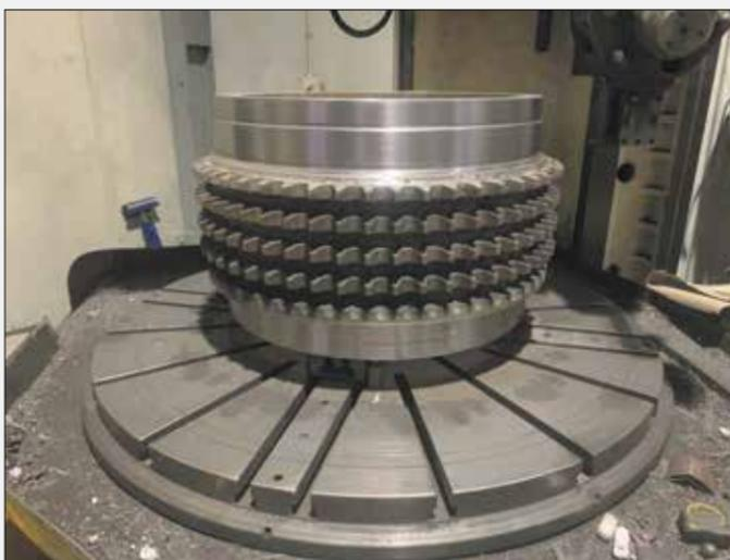
After thermal arc spraying and machining, the bearing surface is fully restored and the part is fit for service once more.
