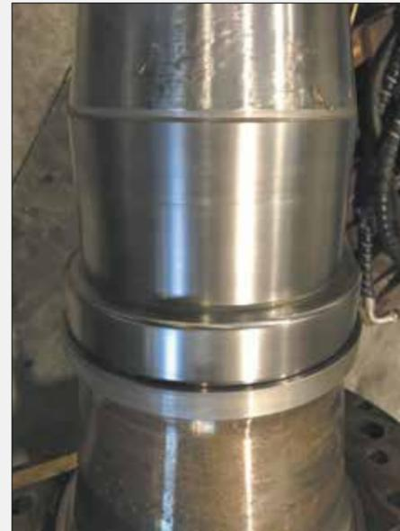
A close-up view of the forklift housing after spraying shows the brand new surface – no trace of the severe scoring it was brought in with.
