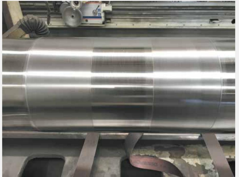
A close-up view of this CAT D10 shaft shows the quality of the finish after thermal arc spraying.
