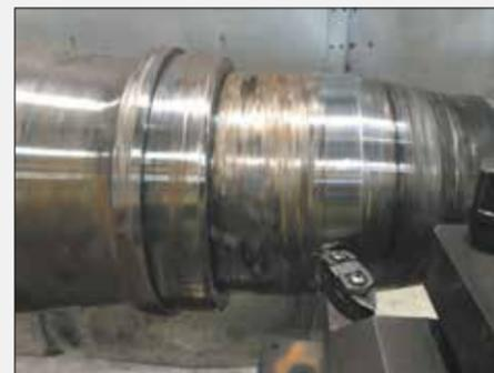
This forklift diff housing was brought in to Arc Spray Engineering for repair, showing signs of extreme wear on the bearing surfaces.
