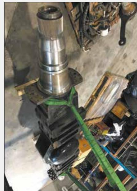
The complete diff housing with newly machined surfaces and a coat of paint – back to work.
